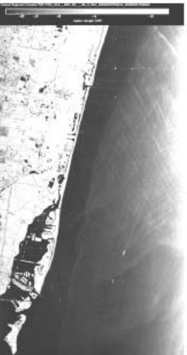
Stripmap, 3 m resolution. Credit to the German Aerospace Center (DLR).
